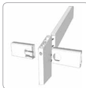
Eaves purlin - exploded view
